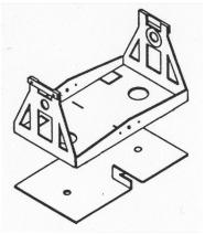
**Step 4.**Fold up the two sides of the units to form a box, and fold up the two locating tabs an the mounting plate, once again with the half etched fold lines on the inside of the bend.
